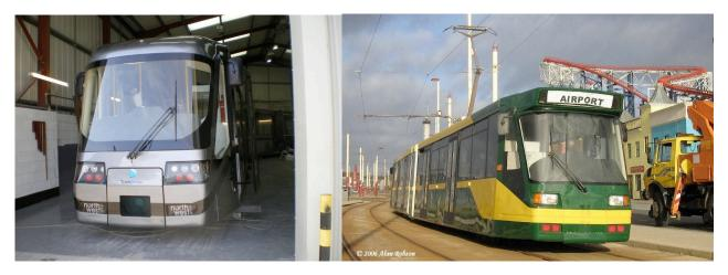
TramPower offers high-specification, high-performance, low-cost and low-energy LRVs. They use 1kWh/km, about one-third of those of our competitors. Independent axles eliminate 'wheel squeal'.
